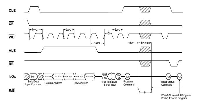
$\textbf{NOTES:} \ \ \textbf{tADL} \ \ \textbf{is the time from the} \ \overline{\textbf{WE}} \ \ \textbf{rising edge of final address cycle to the} \ \overline{\textbf{WE}} \ \ \textbf{rising edge of first data cycle}.$
