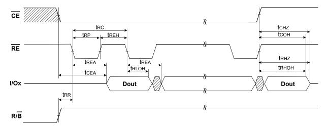
NOTES: Transition is measured ±200mV from steady state voltage with load. This parameter is sampled and not 100% tested. tRLOH is valid when frequency is higher than 33MHz. tRHOH starts to be valid when frequency is lower than 33MHz.
