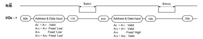
NOTE: It is noticeable that same row address except for A18 is applied to the two blocks
