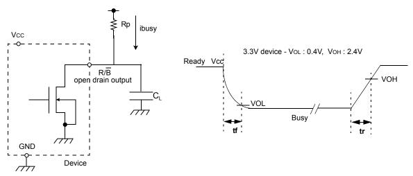
Figure 20. Rp vs tr ,tf & Rp vs ibusy
