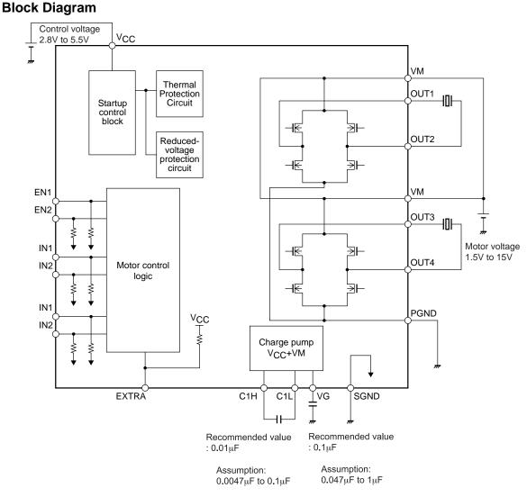
\* Connect a kickback absorption capacitor as near as possible to the IC. Coil kickback may cause increase in VM line voltage, and a voltage exceeding the maximum rating may be applied momentarily to the IC, which results in deterioration or damage of the IC
