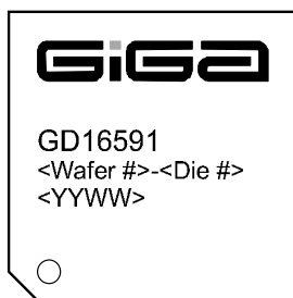
Figure 12. Device Marking - GD16591. Top View.
