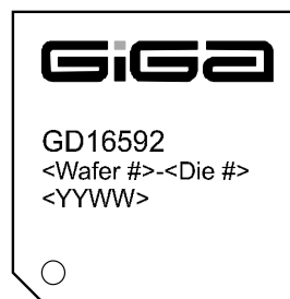
Figure 13. Device Marking - GD16592. Top View.
