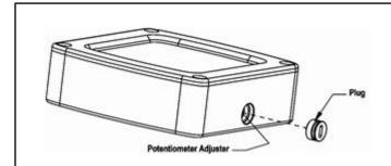
Figure 1. Potentiometer adjuster
