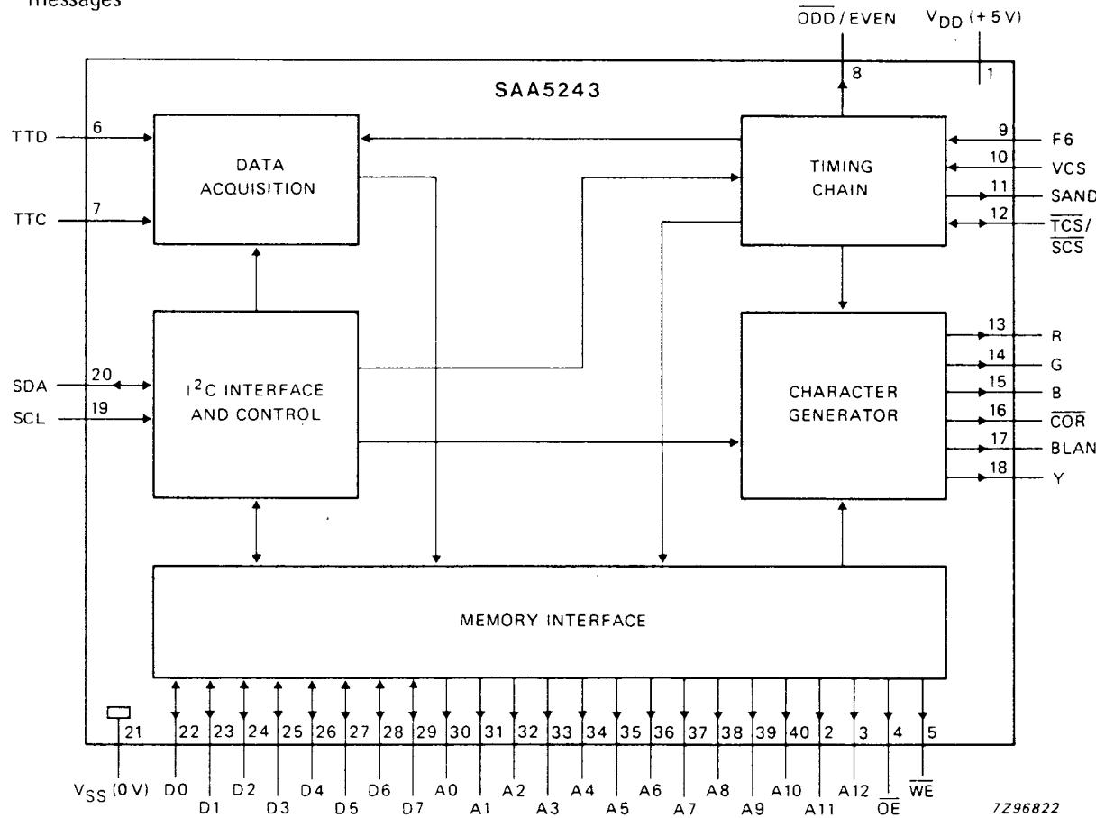
Fig.1 Block diagram.
