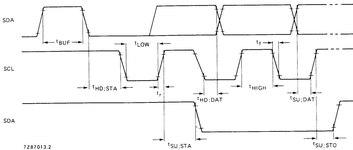
Fig.8 I<sup>2</sup>C-bus timing.
