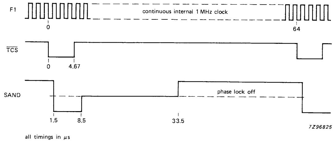
Fig.5 Synchronization timing.
