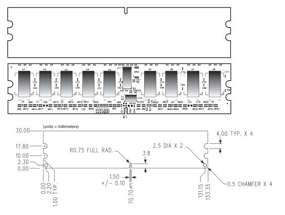
Figure 1: KVR400D2S8R3/1G 240-Pin DIMM
