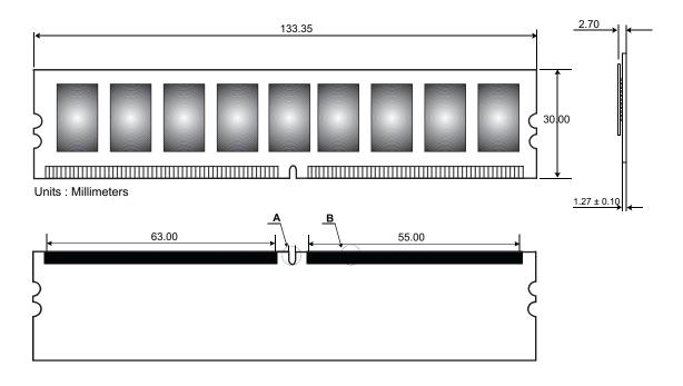
Figure 1: KVR533D2E4/1G 240-Pin DIMM
