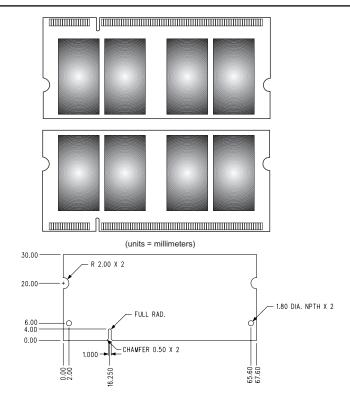
Figure 1: KVR667D2S5/1G 200-Pin SODIMM
