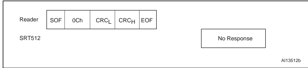
Figure 59. READ_BLOCK frame exchange between Reader and SRT512
