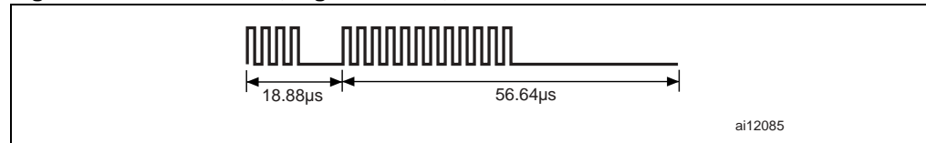
Figure 31. End of frame, high data rate, one subcarrier x2
