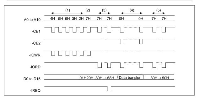
2. Sector write: 1 sector write procedure after the card configured I/O interface is shown as follows.
