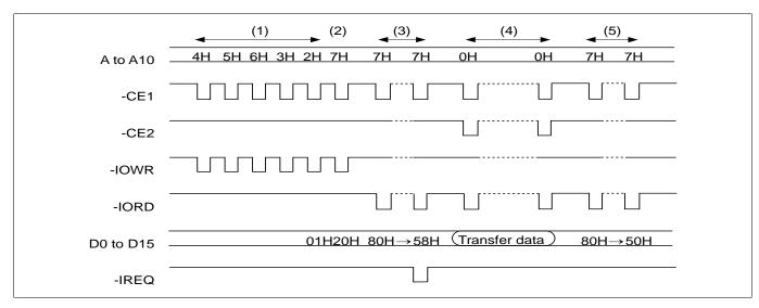
2. Sector write: 1 sector write procedure after the card configured I/O interface is shown as follows.
