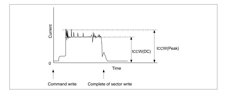
AC Characteristics (Ta = 0 to +60°C,  $V_{CC}$  = 5 V  $\pm$  10%)
