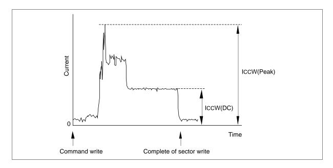
AC Characteristics (Ta = 0 to +60°C,  $V_{CC}$  = 5 V  $\pm$  10%, 3.3 V  $\pm$  5%)
