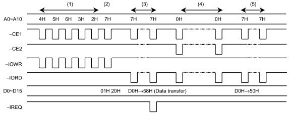
2. Sector write: write sector procedure after the card configured I/O interface is shown as follows.
