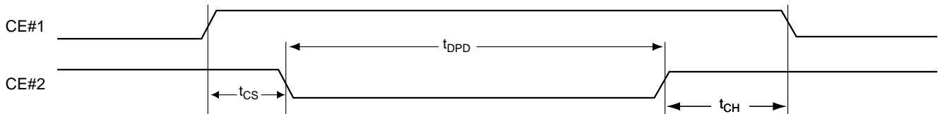
Figure 33. Deep Power-down Timing
