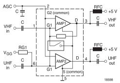
V<sub>GG</sub> = 5 V: UHF AMP is on; VHF AMP is off V<sub>GG</sub> = 0 V: UHF AMP is off; VHF AMP is on (0 = shorted to Ground or open)
