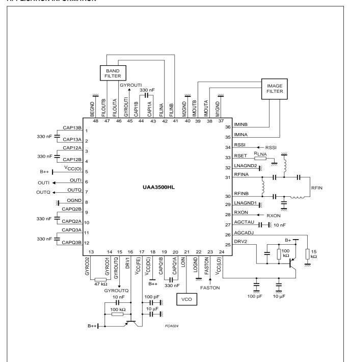
Electrical diagram of the UAA3500HL demonstration board for FLEX<sup>TM</sup> applications. All matching is to 50  $\Omega$  for measurement purposes. B+ = 1.4 V; B++ = 2.1 V.
