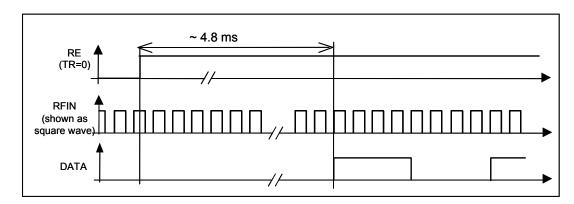
The carrier detector set-up time (after TR bit set to 0 and RE input set to 1) is 4.85ms when the carrier frequency is 36.86 kHz. In the applications where the carrier detector is turned on for a relative long period (tens to hundreds of ms), it is recommended to reset the block with a short transition to stand-by mode (RE=0).
