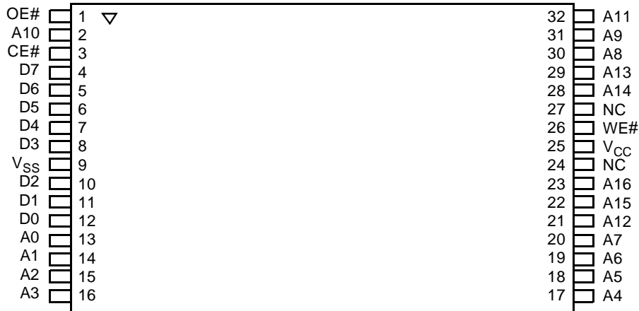
32-Pin TSOP—Reverse Pinout
