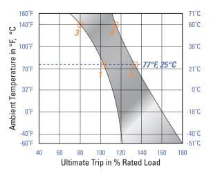
Performance characteristics are based on room temperature (77°F, 25°C). Consult Denating curve for ambient temperatures significantly higher or lower than standard room temperature.
