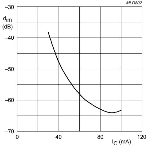
$V_o = 700$  mV;  $V_{CE} = 12$  V;  $T_{amb} = 25$  °C;  $f_{(p+q+r)} = 793.25$  MHz.
