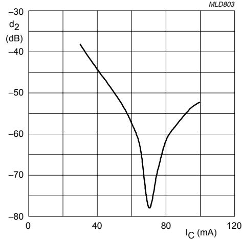
$V_o = 316$  mV;  $V_{CE} = 12$  V;  $f_{(p+q)} = 810$  MHz.
