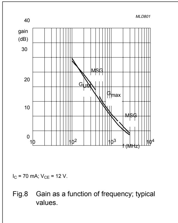
Fig.8 Gain as a function of frequency; typical
