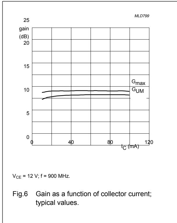
Fig.6 Gain as a function of collector current;
