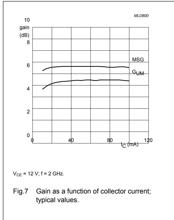
Fig.7 Gain as a function of collector current;
