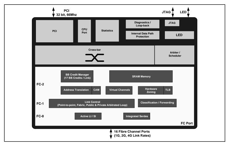
The BCM8440 Fibre Channel Fabric Switch IC offers a high level of system integration, performance and features for next generation Fibre Channel switches. Because of the small form factor and low power the BCM8440 is ideal for embedded Fibre Channel Fabric Switch applications or cost effective stand-alone switches.
