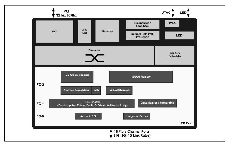
The BCM8441 Fibre Channel Fabric Switch IC offers a high level of system integration, performance and features for next generation Fibre Channel switches. Because of the small form factor and low power the BCM8441 is ideal for embedded Fibre Channel Fabric Switch applications or cost effective stand-alone switches.
