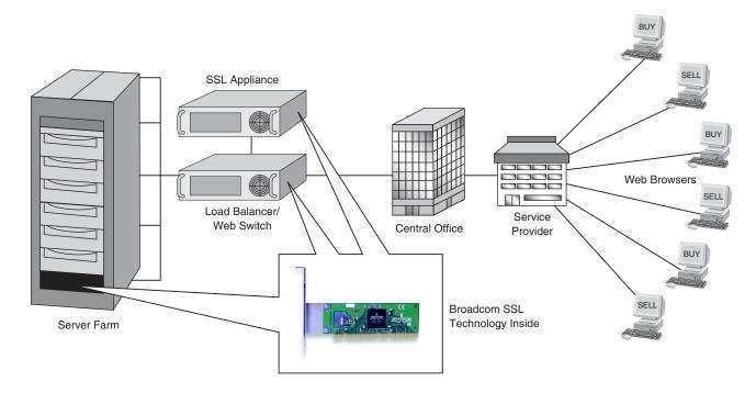
Broadcom's **SSL1600** accelerator adapter is a complete highperformance SSL accelerator designed to accelerate the public-key cryptographic functions of SSL, thereby freeing the host CPU. This results in a dramatic improvement in the overall performance of the host system, drastically reducing CPU utilization and enabling additional CPU bandwidth for other value-added services and features.
