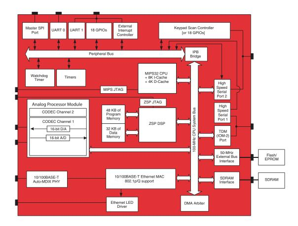
Broadcom's BCM1115 is designed for use in cost-sensitive, single Ethernet port consumer and Enterprise IP Phone and Gateway products.
