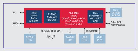
Small Form Factor 48 + 2G Layer 2 Ethernet over VDSL Switch **Application Example**
