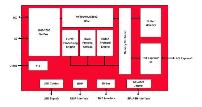
The BCM5708S provides a fully integrated Layer 4 and Layer 5 solution – TCP/IP, RDMA, and iSCSI along with a complete 1000/2500BASE-X Gigabit Ethernet, IEEE 802.3<sup>™</sup> compliant Media Access Control (MAC), and Physical Layer Transceiver solution for high performance network applications. By itself, the BCM5708S provides a complete single-chip Gigabit Ethernet NIC with a TCP/IP Processing Engine, RDMA NIC (RNIC), iSCSI HBA, or LOM solution.
