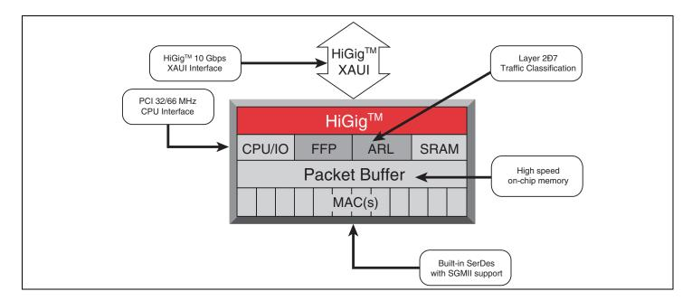
The BCM5690 network switch is a scalable, modular chip solution with 12 ports. Each of these flexible ports supports Gigabit Ethernet or 10/100 Mbps Ethernet. Additionally, the BCM5690 supports both copper and fiber physical interfaces. The BCM5690 has a fully integrated SerDes functionality consisting of a 10 Gbps XAUI HiGig Port, Gigabit Ethernet or a SGMII PHY interface.
