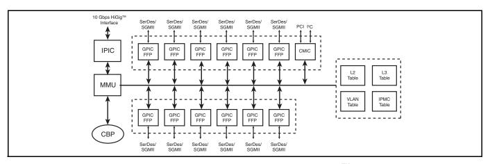
12-Port Gigabit Ethernet Multilayer Switch with HiGig™
