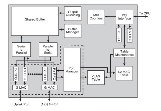
The BCM5633 switching processor chip supports 13-Gigabit ports with all ports in wirespeed operation. The BCM5633 is ideal for applications such as multi-Gigabit port switches or aggregating multiple-Gigabit ports.
