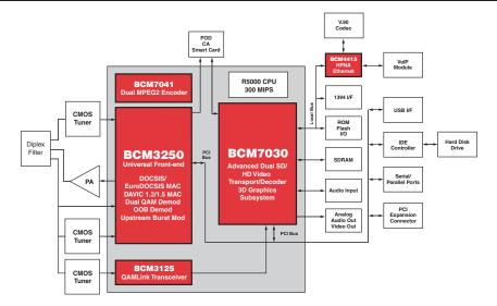
The Broadcom **BCM93740** is an advanced set-top box development platform supporting high definition television (HDTV), dual standard definition decoding and broadband cable modem internet access. It is a highly integrated, cost-effective design built on the latest generation of Broadcom silicon and software offering low risk and quick time-to-market for the next generation of interactive set-top boxes.
