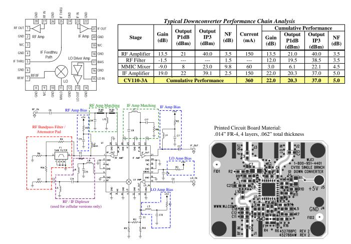
**CV110-3A**: The application circuit can be broken up into four main functions as denoted in the colored dotted areas above: RF/IF diplexing (purple), amplifier matching (green), filtering (red), and dc biasing (blue). There are various placeholders for chip components in the circuit schematic so that a common PCB can be used for all WJ single-branch converters. Additional placeholders for other optional functions such as filtering are also included.
