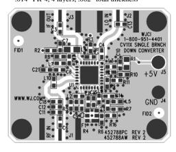
**CV110-1A**: The application circuit can be broken up into four main functions as denoted in the colored dotted areas above: RF/IF diplexing (purple), amplifier matching (green), filtering (red), and dc biasing (blue). There are various placeholders for chip components in the circuit schematic so that a common PCB can be used for all WJ single-branch converters. Additional placeholders for other optional functions such as filtering are also included.
