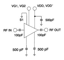
1. Self-bias operation is obtained by connecting +6 volts to both VDD and VDD pads, grounding pad S1, and connecting pads GND1 and GND2 to separate bypass 500pF MOS capacitors.
