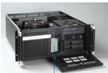
Easy-to-maintain system fan & reusable filter
