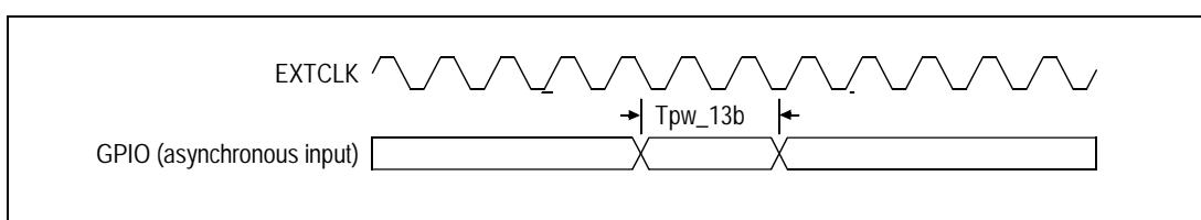
Figure 5 GPIO AC Timing Waveform
