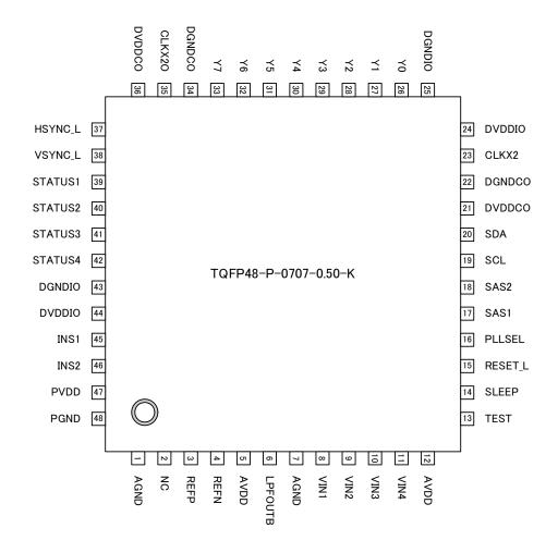
48-Pin Plastic TQFP (TQFP48-P-0707-0.50-K)
