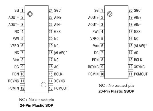
\* The ALAW pin is only applied to the MSM7507-01GS-K/MSM7507-01MS-K.
