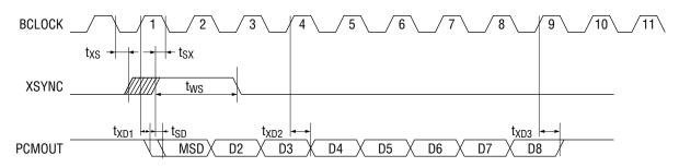
When  $t_{XS} \le 1/2 \bullet Fc$ , the Delay of the MSD bit is defined as  $t_{XD1}$ . When  $t_{SX} \le 1/2 \bullet Fc$ , the Delay of the MSD bit is defined as  $t_{SD}$ .
