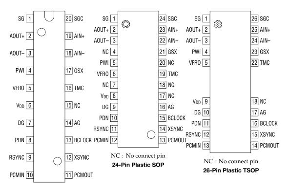
NC : No connect pin **20-Pin Plastic Skinny DIP**
