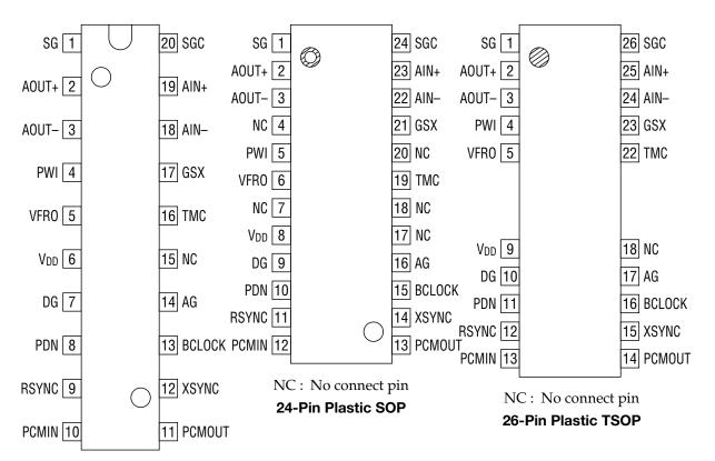
NC : No connect pin **20-Pin Plastic Skinny DIP**
