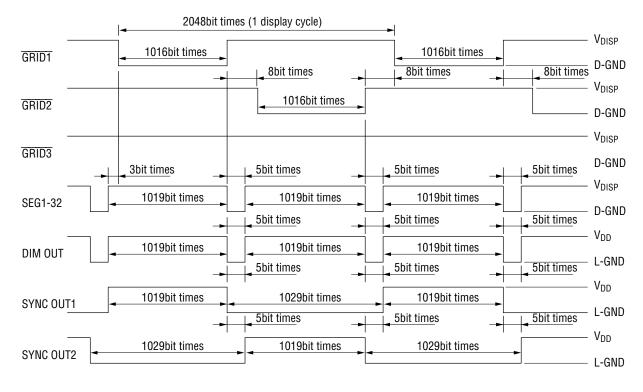
• Output Timing (Triplex Operation) \*1bit time=4/f<sub>OSC</sub> (The dimming data is 1016/1024 at the master mode)
