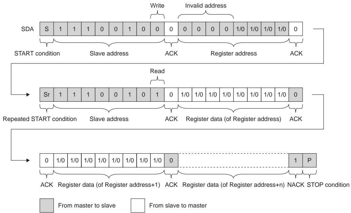
When the master returns ACK (0 data) after reading of the initial register • address • data of read sequence, the register • address increases by one address, enabling consecutive reading of data corresponding to each register address. If the master does not return ACK (0 data), the register address does not increase.
