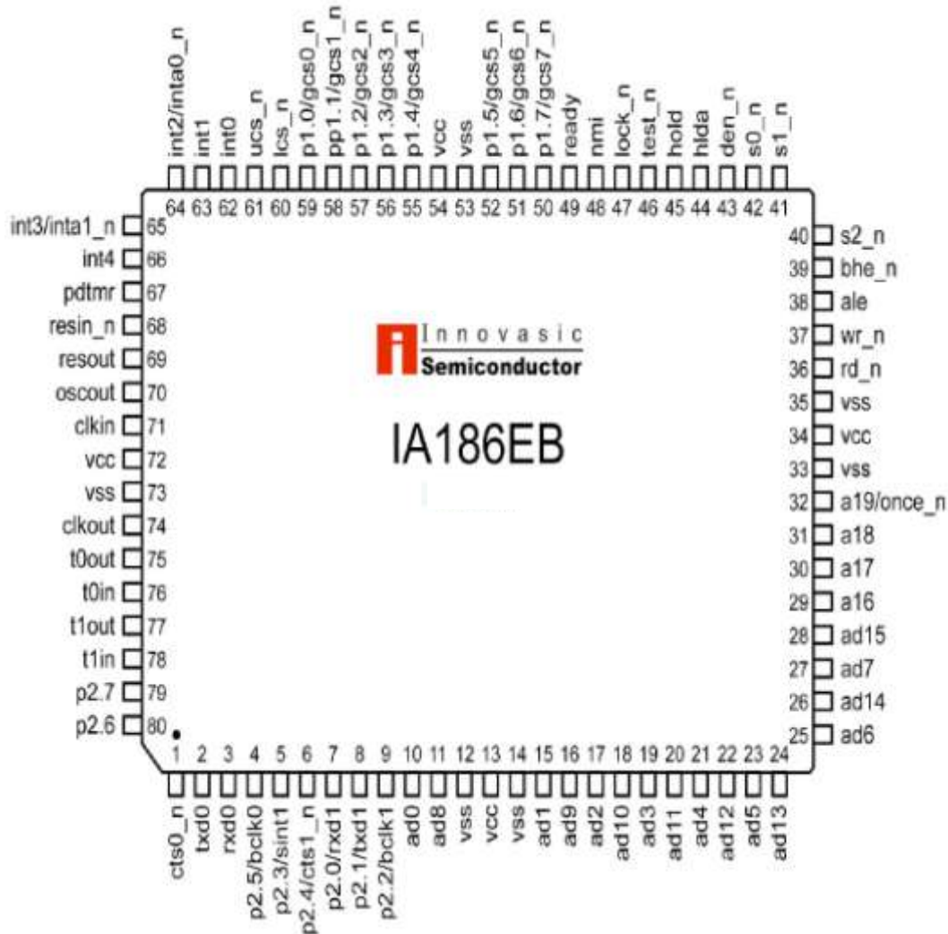
Figure 4. IA186EB 80-Pin PQFP Package Diagram
