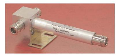
Microlab Model Dx-82FN series of 2, 3 and 4 way Power Splitters has been designed to evenly split PCS, UMTS, WiFi and WiMAX signals with minimal reflections or loss. All joints are moisture sealed with 'O' rings to meet IP67. The mechanical shape allows easy attachment to wall using the supplied bracket.
