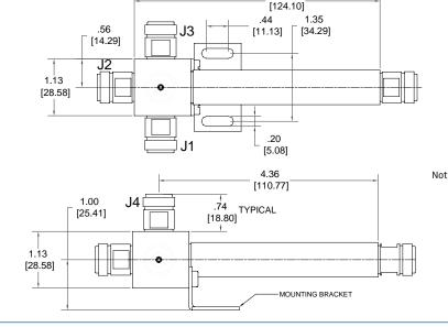
D2-82FN 2 way Splitter delete J2 & J4 D3-82FN 3 way Splitter delete J4 D4-82FN 4 way Splitter as drawn.
