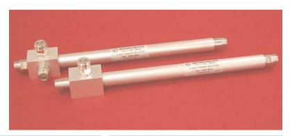
Microlab Model Dx-86FN series of 2, 3 and 4 way Power Splitters has been designed to evenly split high power cellular and WiMAX signals with minimal reflections or loss. All joints are moisture sealed to meet the IP67. The mechanical shape allows easy attachment to wall using the supplied clip and bracket.
