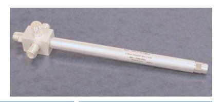
Microlab Model Dx-88FN series of 2, 3 and 4 way Power Splitters has been designed to evenly split high power cellular signals with minimal reflections or loss. All joints are moisture sealed to meet the IP67 rating. The mechanical shape allows simple attachment to wall using the supplied clip and bracket.
