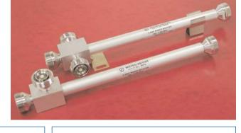
Microlab Model Dx-88FD series of 2, 3 and 4 way Power Splitters has been designed to evenly split high power cellular signals with minimal reflections or loss. All joints are moisture sealed to meet the IP67 rating. The mechanical shape allows simple attachment to wall using the supplied clip and bracket.
