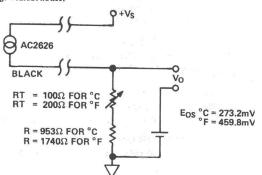
For most applications, a single point calibration is sufficient. With the probe at a known temperature, adjust  $R_{\rm T}$  so that  $V_O$  corresponds to the known temperature.
