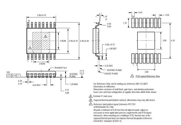
Package LP, 16-Pin TSSOP with exposed thermal pad
